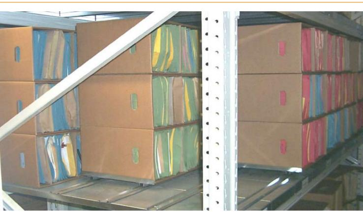
In a two deep shelf layout the boxes are stowed 4, 5 and 6 in the width depending on the box size and available beam length, and by 2 and 3 high in the height.
